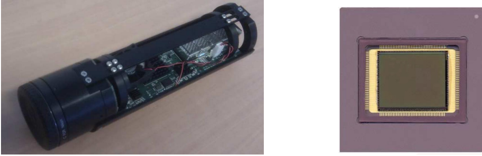
Figure 1.11. Camera head and image sensor.
