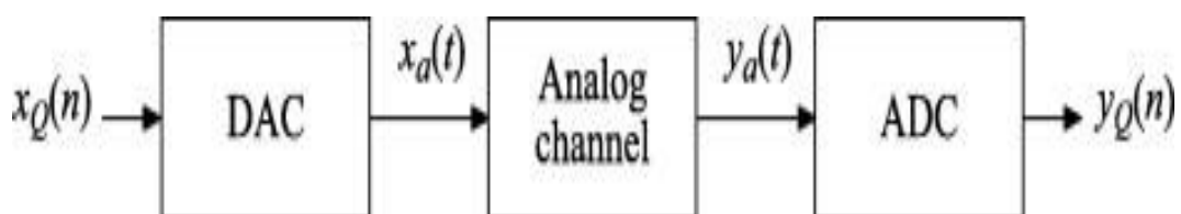
Figure 2. Simplified model of digital communication system [2]
