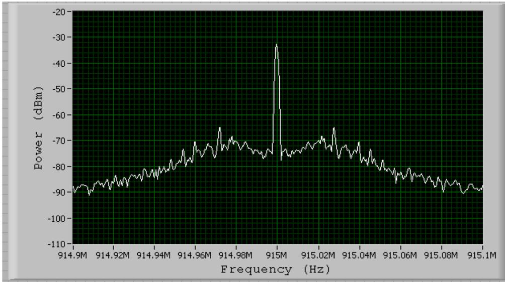
**Fig. 4.5: Power Spectrum of TRF6900A output signal with corrected frequency**
