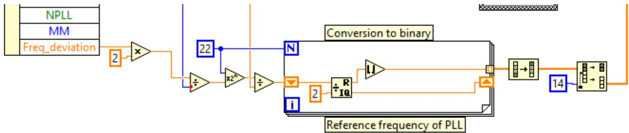
Fig. 4.14: Conversion of the frequency deviation to binary in codeword D
