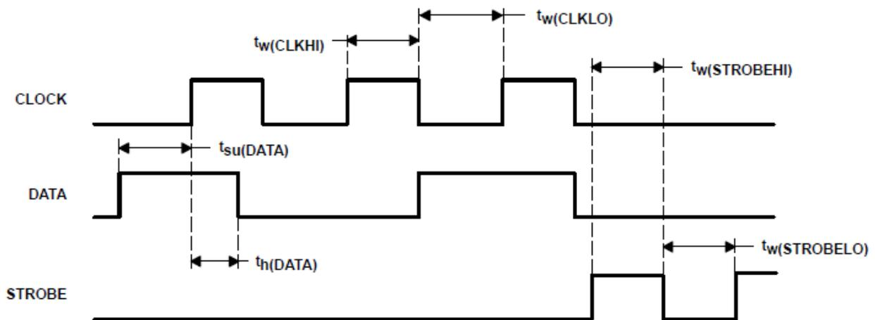
Fig. 3.6: TRF6900A serial interface timing diagram
