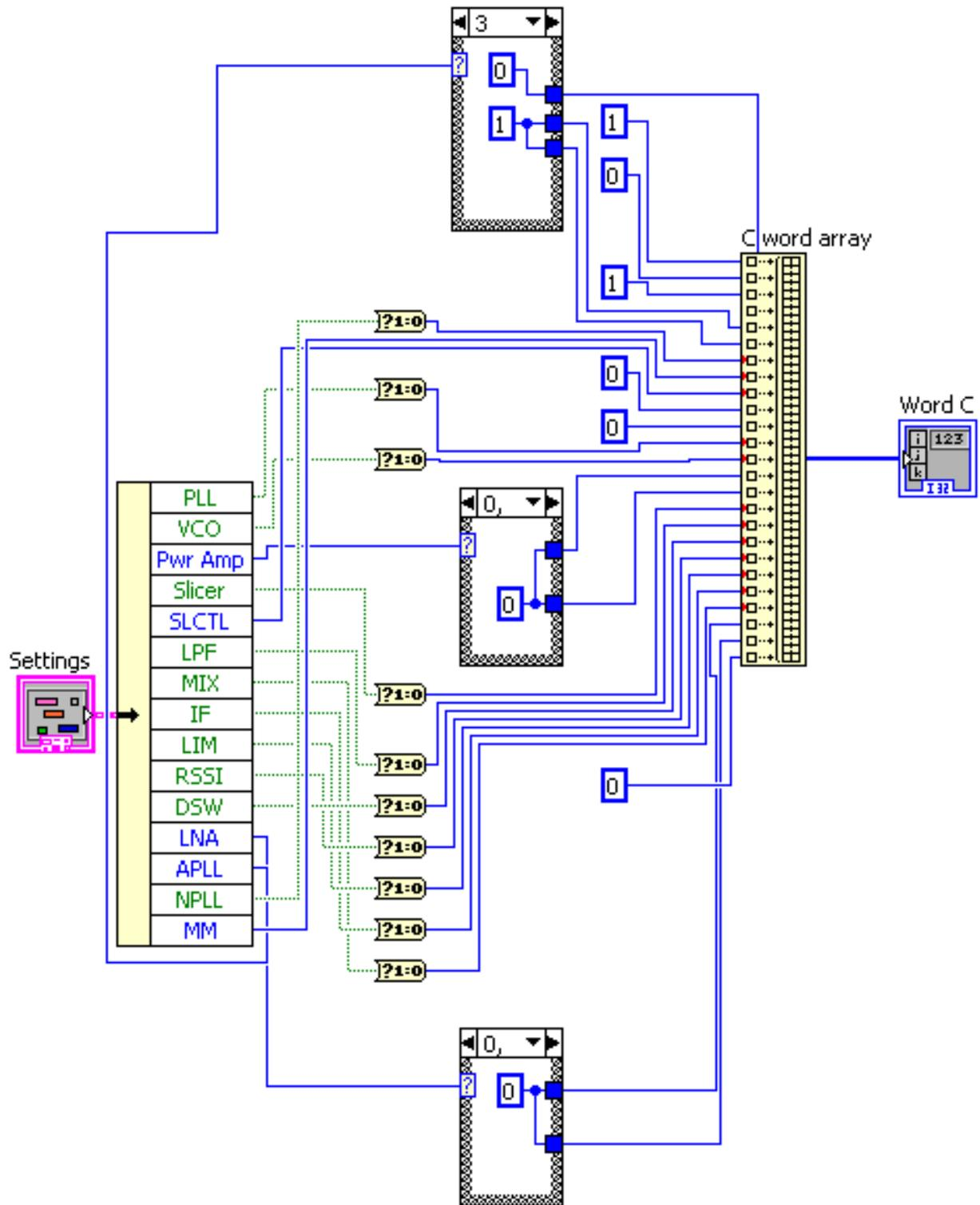
Fig. 0.3: Block diagram for codeword C
