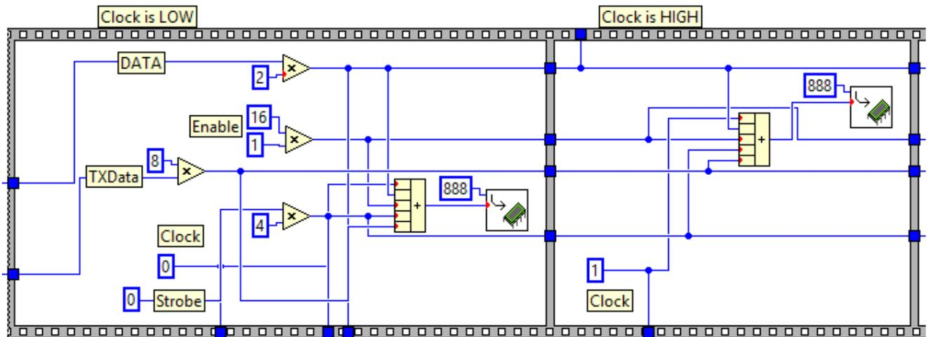
**Fig. 3.11: Communication setup for custom control of TRF6900A**
