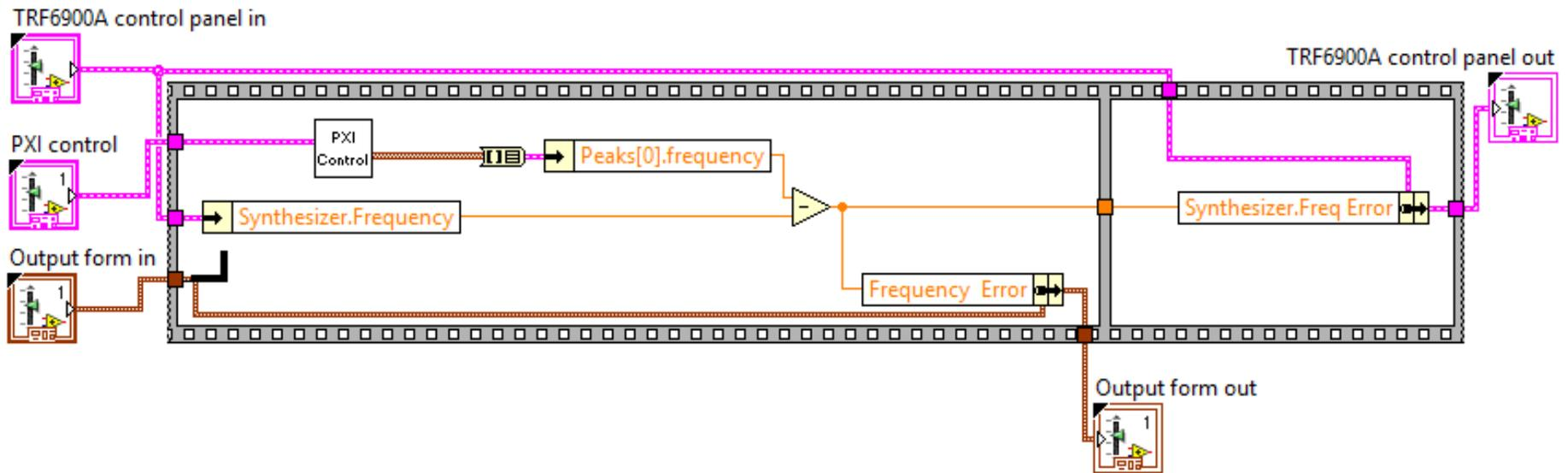
Fig. 4.6: Error detection and correction
