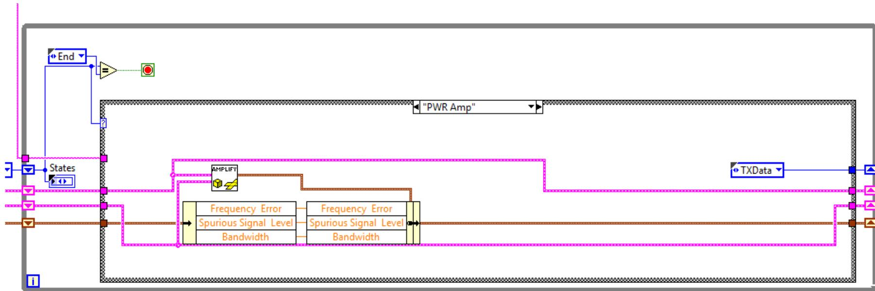
Fig. 0.20: Power amplifier state in the automated testing system
