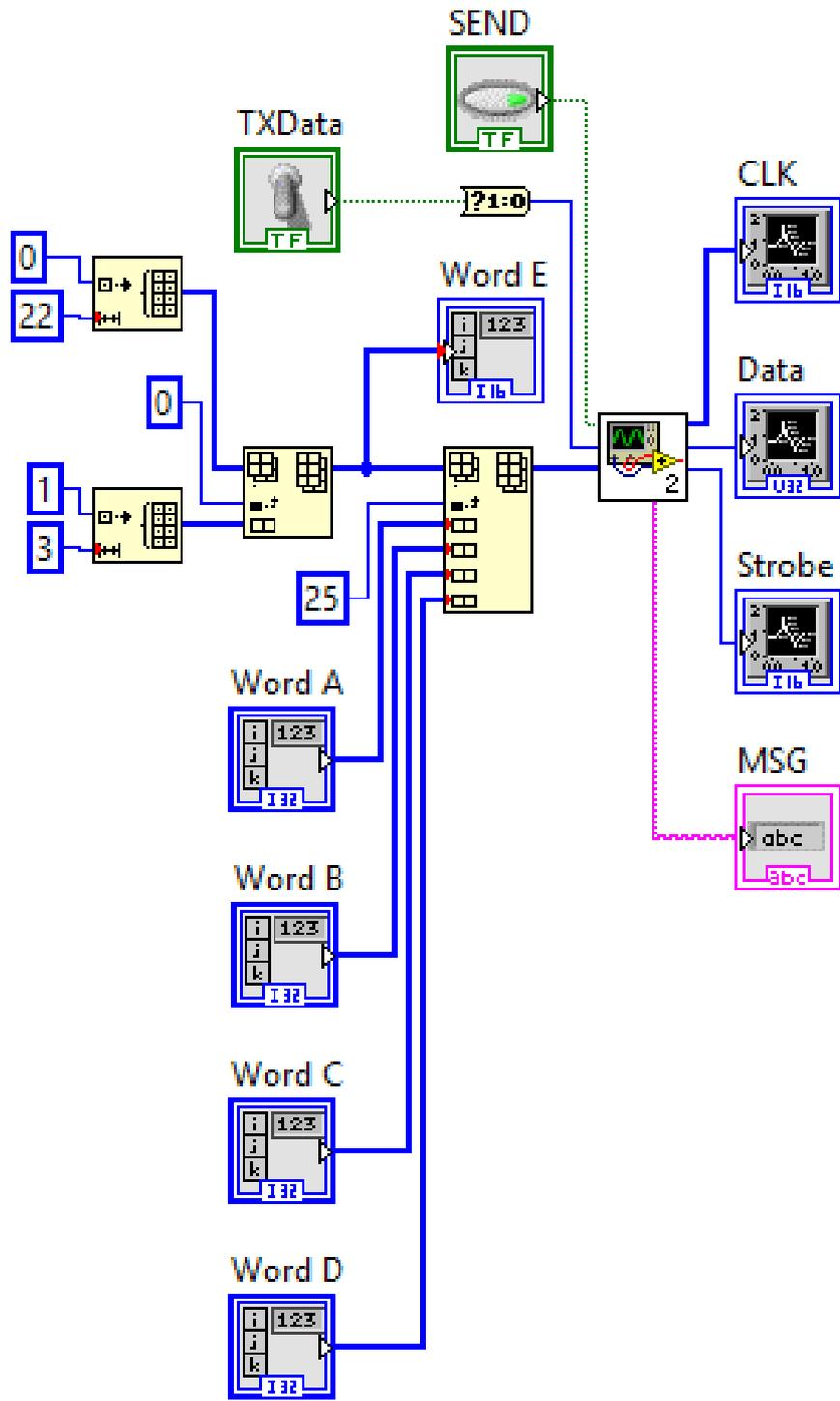
Fig. 0.5: Block diagram for TRF6900AA communication
