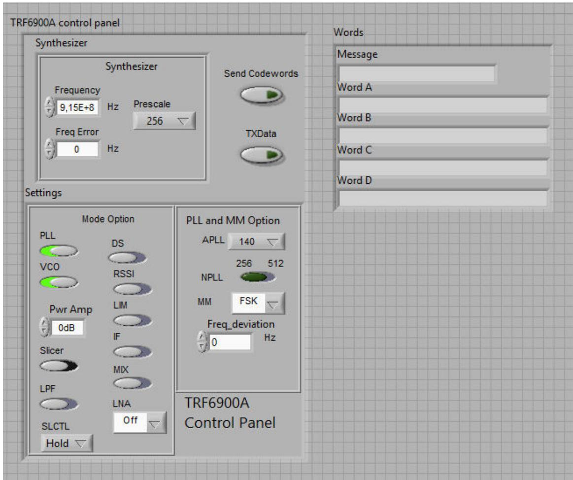
Fig. 0.1: User interface for TRF6900A custom control
