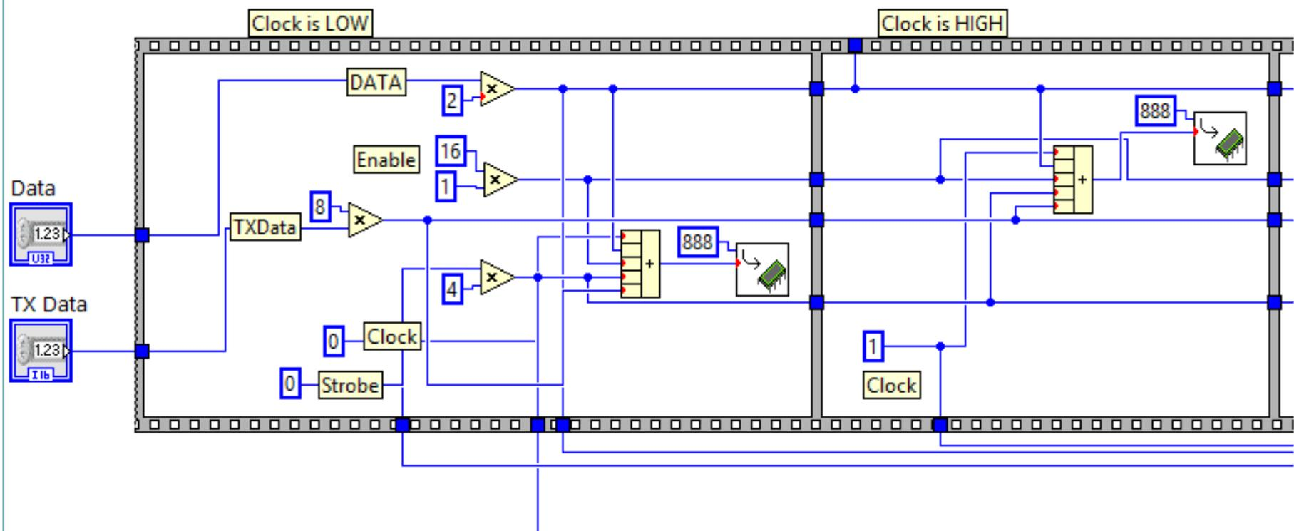
Fig. 0.7: Codeword sending state with clock Low-High-High-Low (part a)
