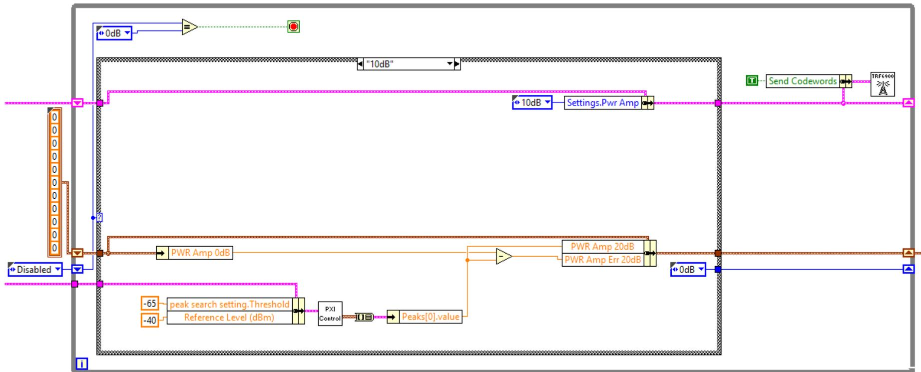
In the case structure, PXI measures current signal level, while the trf board is set for the next level
