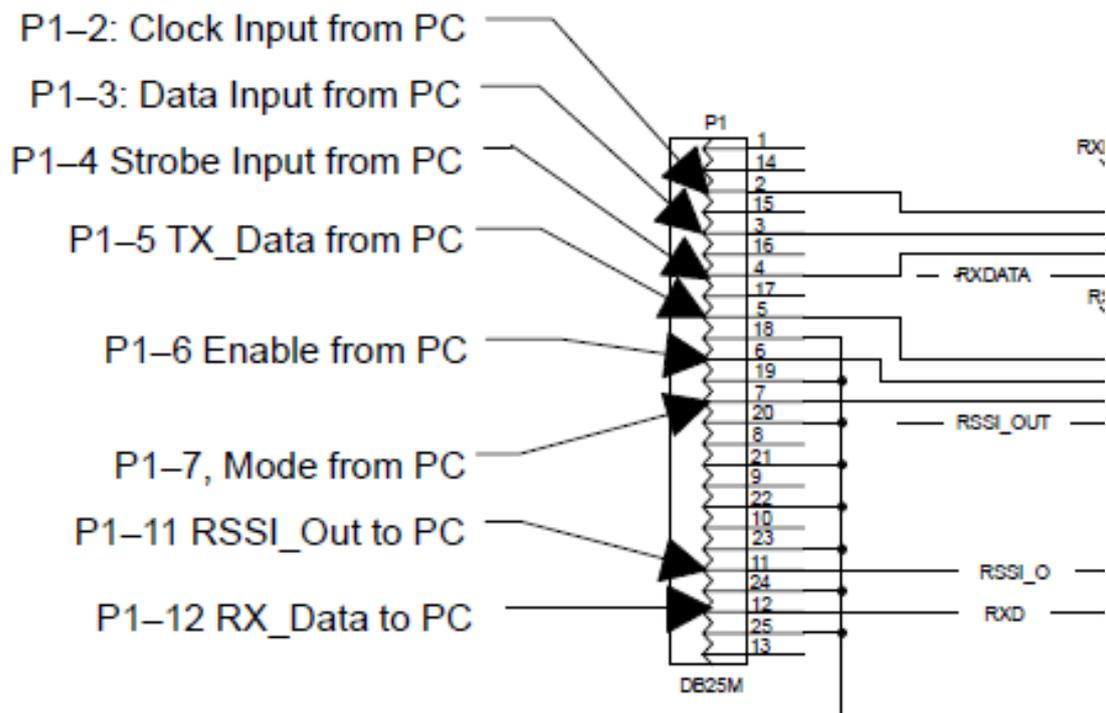
**Fig. 4.15: Parallel port pins used for serial interface of TRF6900AA control**
