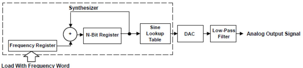
Fig. 3.5: Typical DDS Block Diagram
