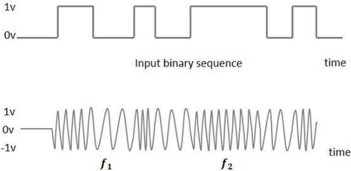
**Fig. 4.12: FSK modulated output wave**
