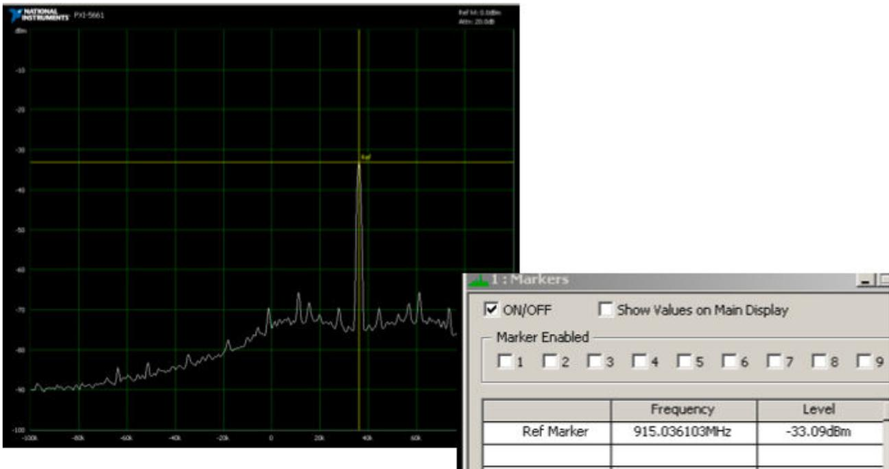
**Fig. 4.4 : Power Spectrum of the TRF6900A output signal before correction**
