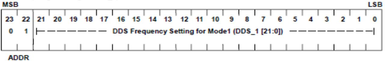
**C-Word (Control Register for PLL, Data Slicer and Mode1 Settings)**
