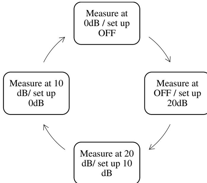
**Fig. 4.10: Measurement states for power amlifier settings**
