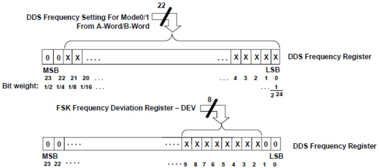
Fig. 4.13: Implementation of the DDS frequency and FSK deviation in the DDS frequency register
