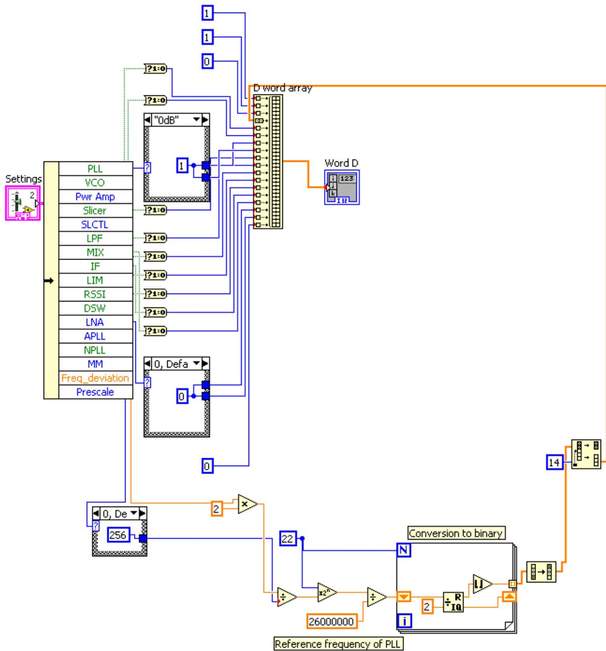
Fig. 0.4: Block diagram for codeword D
