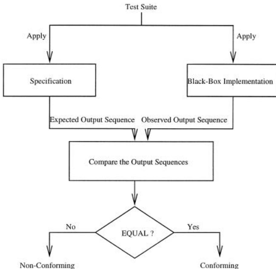
**Fig. 2.1: Conformance testing principle**
