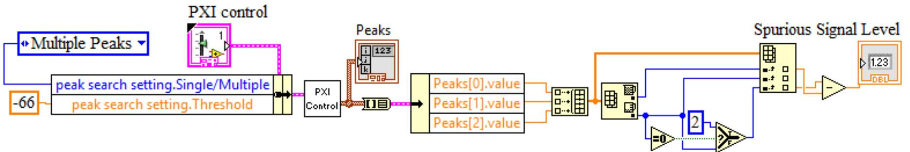
Fig. 4.7: Spurious signal level detection
