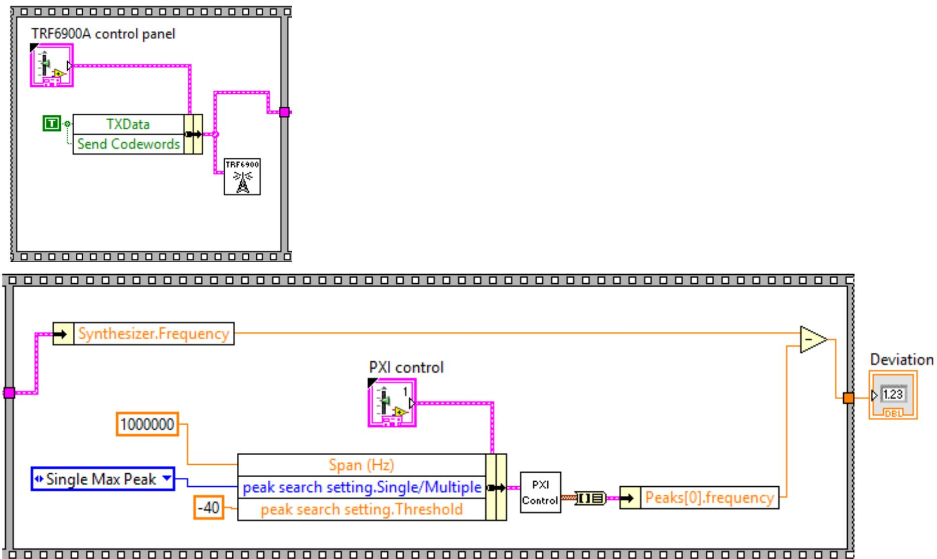
Fig. 4.16: FSK frequency deviation block diagram
