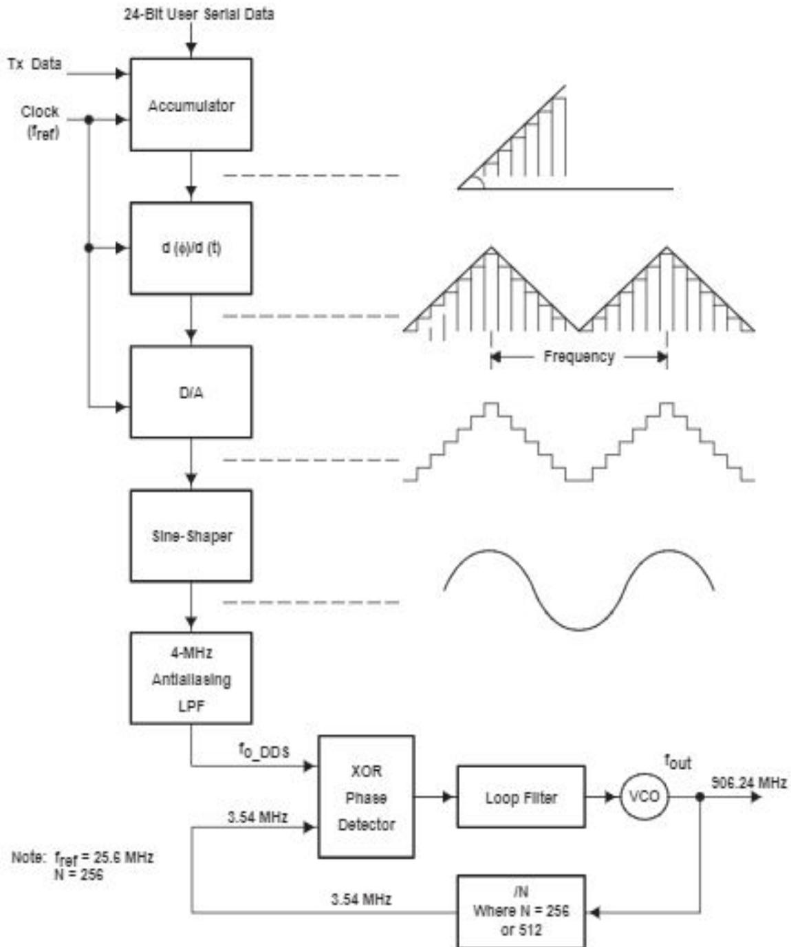
Fig. 4.3: TRF6900A DDS/Synthesizer block diagram
