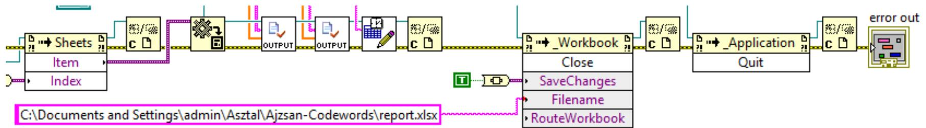
Fig. 0.29: Block diagram for report generation (part c: save the report and close Excel application)
