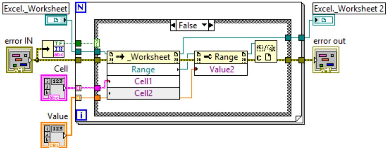
**Fig. 4.18: Cell modification for test report**
