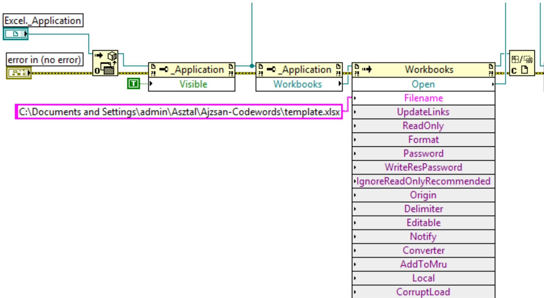
Fig. 0.27: Block diagram for report generation (part a: open the template)
