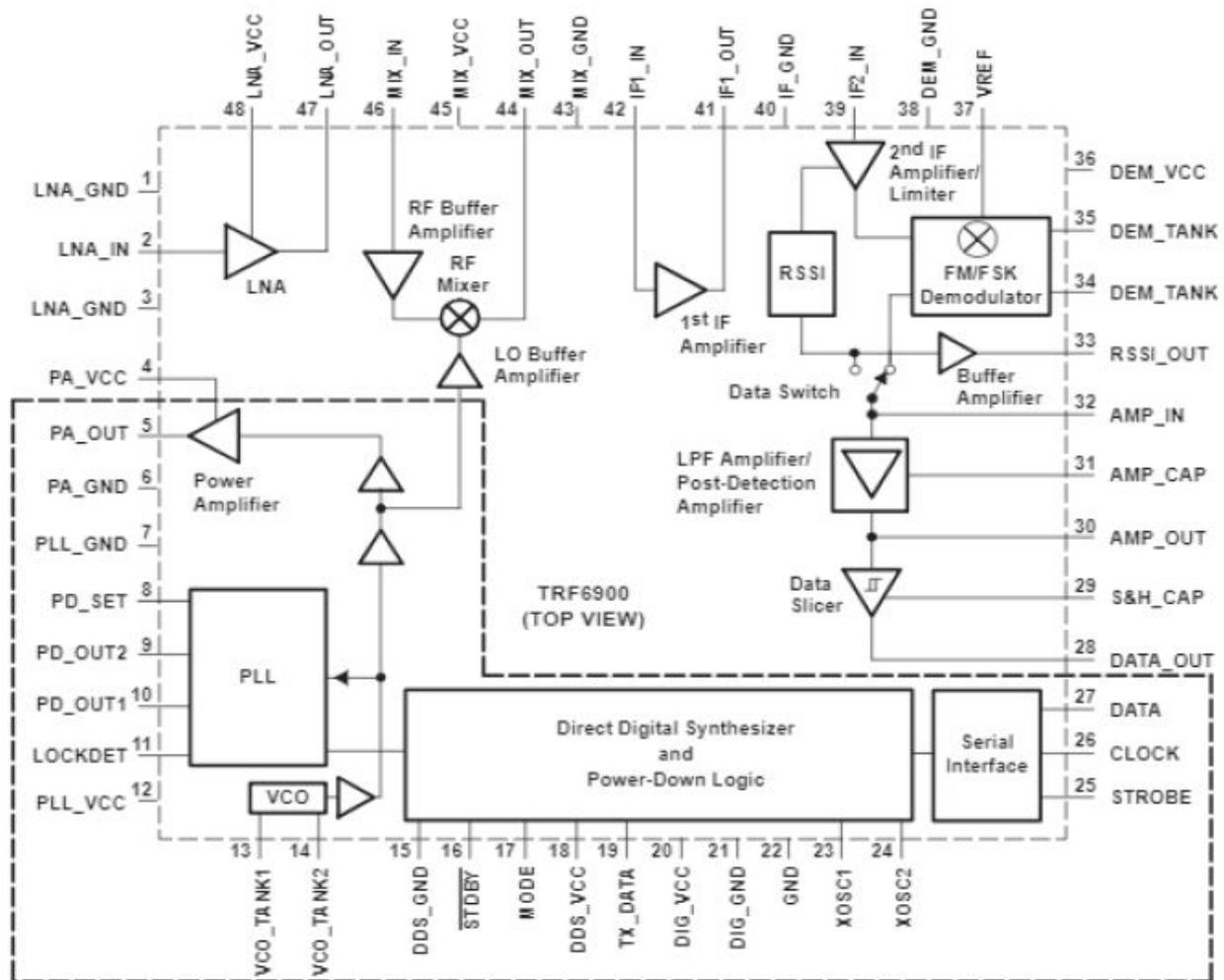
Fig. 3.4: Chip layout of TRF6900A transceiver [7] with dashed area representing transmitter
