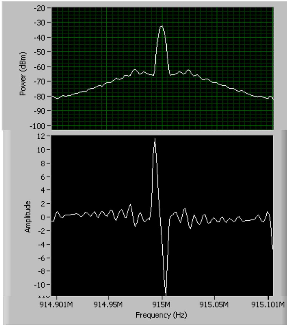
**Fig. 4.8: Signal power spectrum and its derivative**
