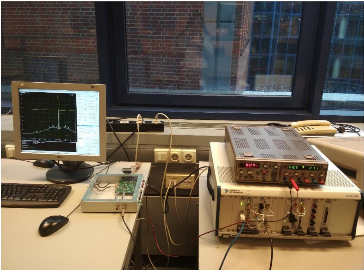
**Fig. 3.1: Equipment setup for the testing system from left to right: control computer, TRF6900A transmitter, power supply and PXI Chassis**
