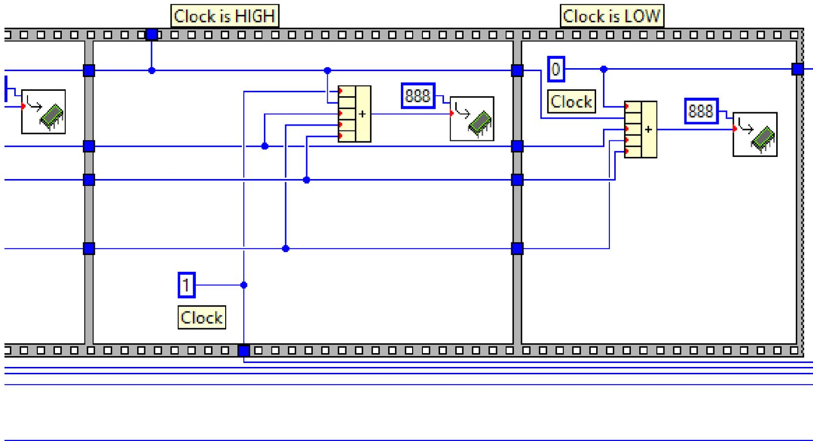
Fig. 0.8: Codeword sending state with clock Low-High-High-Low (part b)
