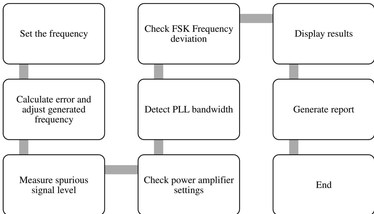
Fig. 4.1: The automated testing system for TRF6900A transmitter
