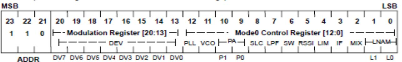
**Fig. 3.8: Codeword for TRF6900A control**
