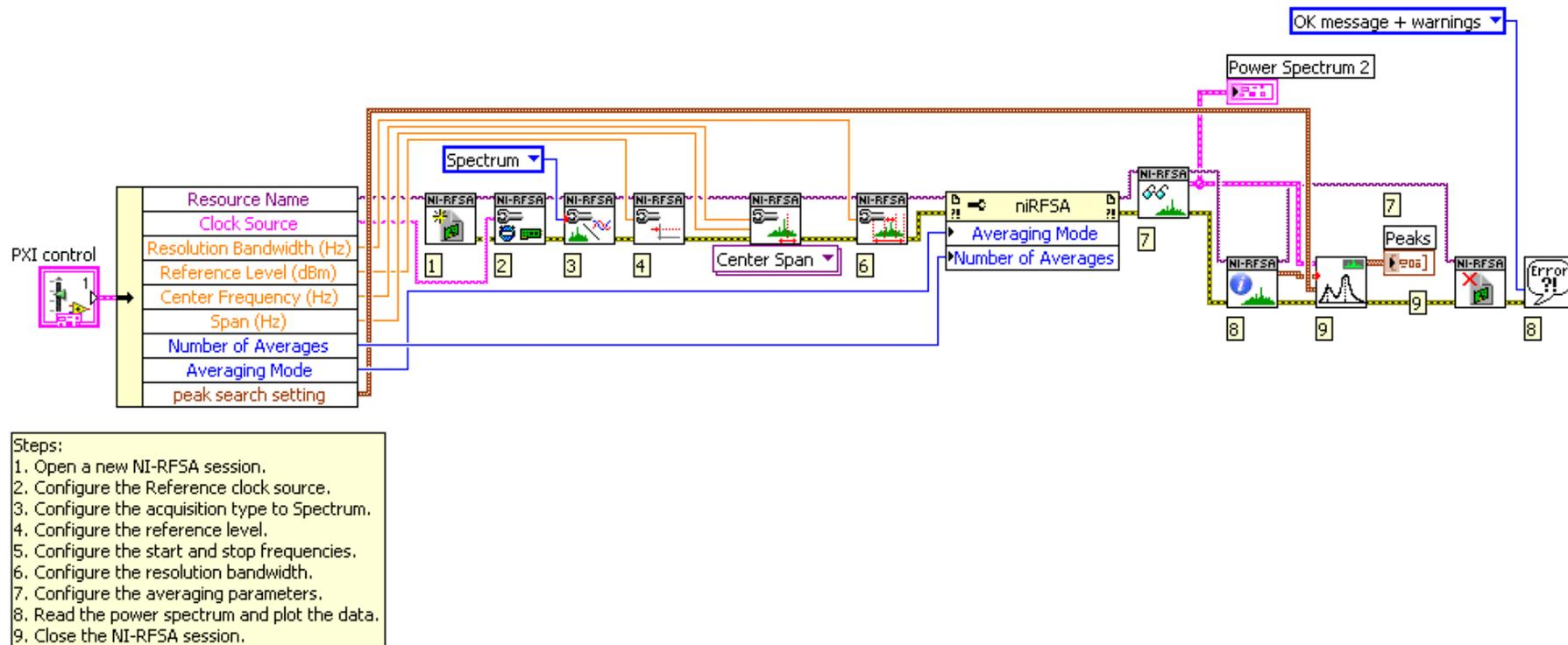
Fig. 0.13: PXI control block diagram
