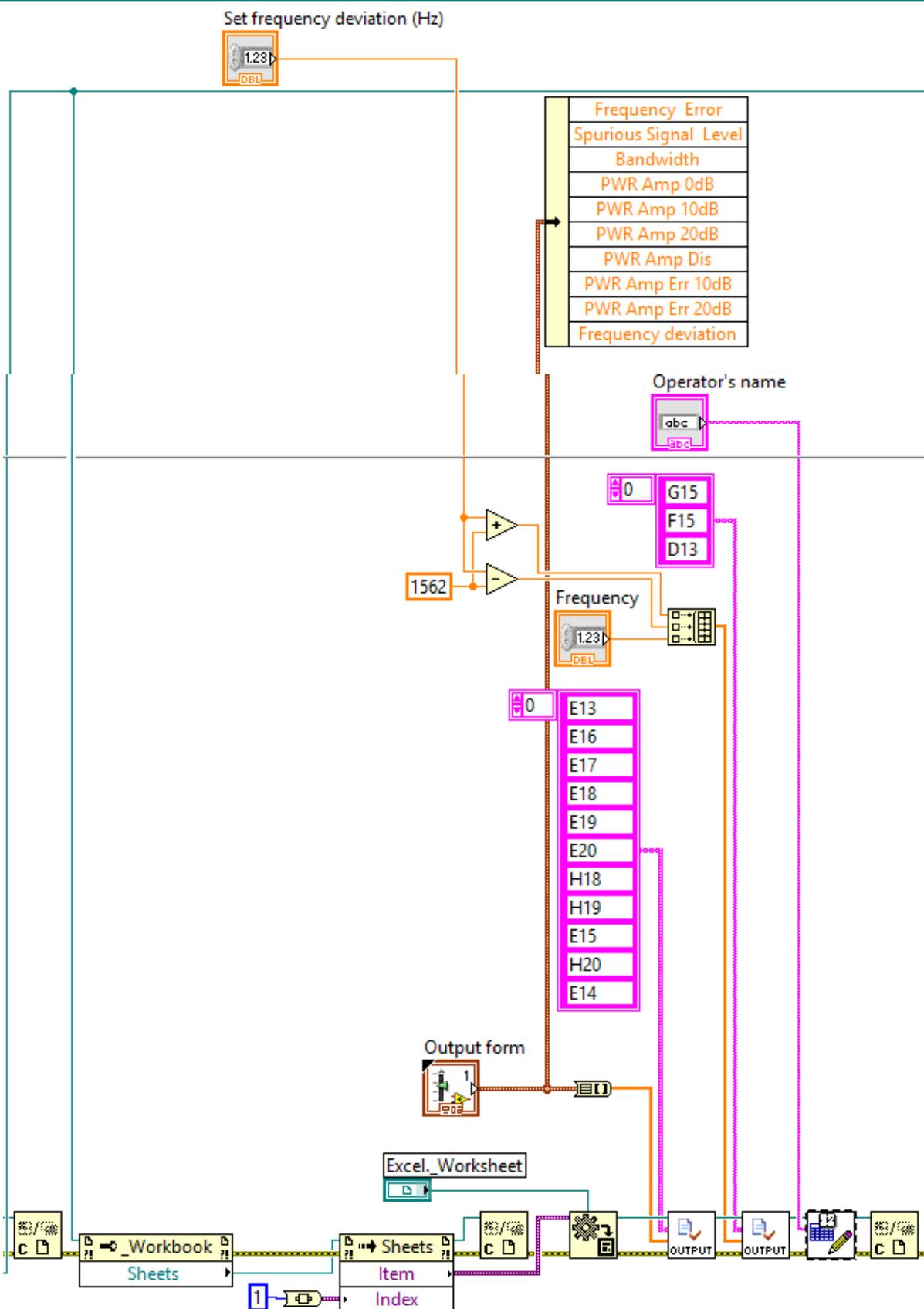
Fig. 0.28: Block diagram for report generation (part b: modify the template)
