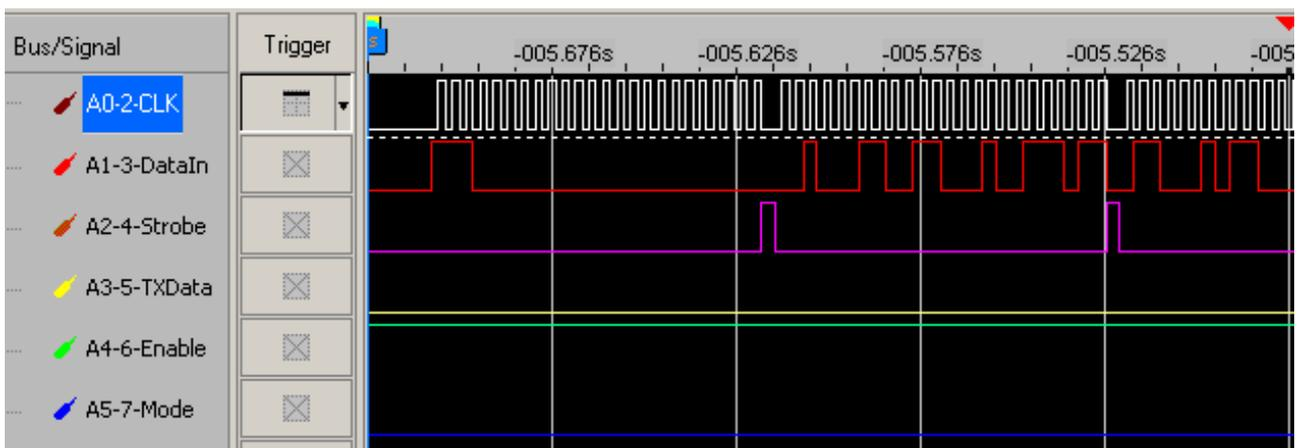
**Fig. 3.10: Control signals on parallel port for TRF6900AA transmitter**
