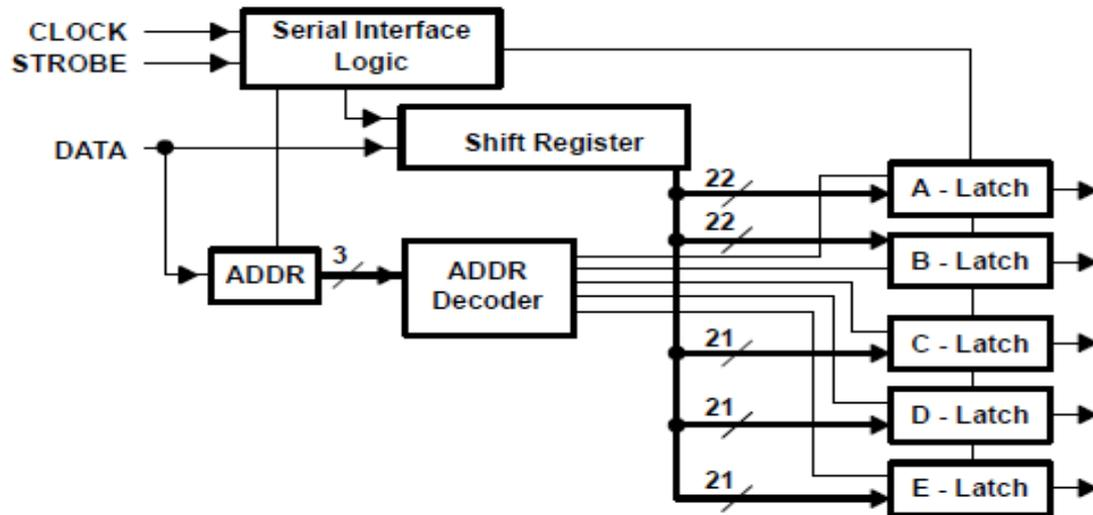
Fig. 3.7: Decoding input signals of TRF6900A
