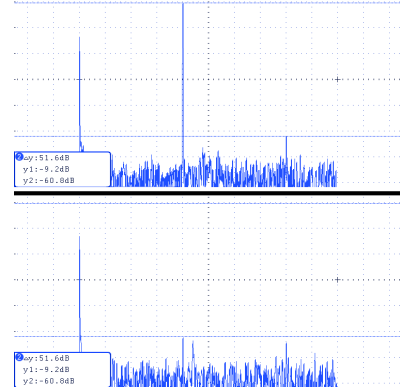
Fig. 8. Output spectrum without (top) and with (bottom) the controller in operation. Horizontal scale 25 kHz/div.
