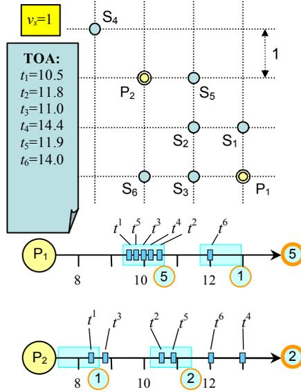
Figure 1. Illustration of the consistency function concept in 2D for a single event. The values of the consistency function are calculated at positions  $P_1$  and  $P_2$  from sensor data  $t_1, t_2, \dots, t_6$ . The true position is  $P_1$  and the emission time is 10.
