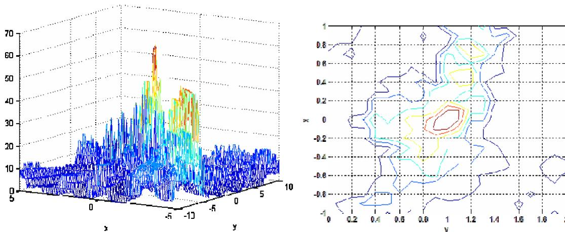
Figure 5. Result of the localization process. The maximum value of the consistency function is 62. The true location was at  $x=0$ ,  $y=1$ , which is detected with 0.2m accuracy.
