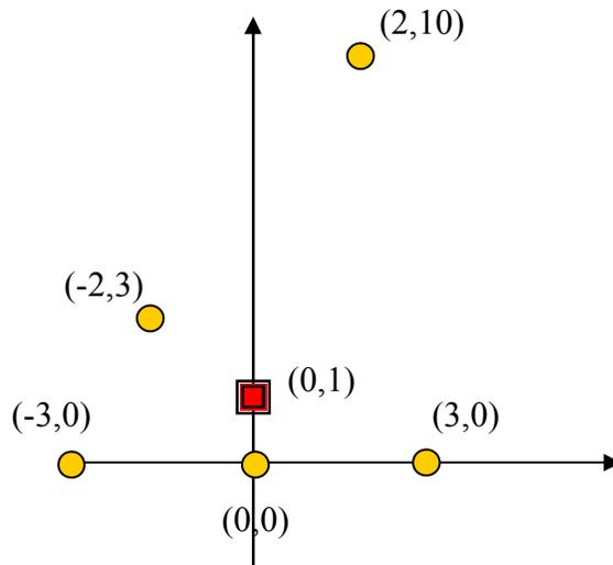
Figure 3. Experimental layout for testing the acoustic localization system containing 5 microphones (circles) and a source (square).
