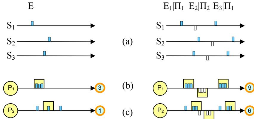
Figure 2. Comparison of the original (left) and the generalized (right) consistency functions: (a) events shown at each sensor's timeline, (b) consistency calculated at the correct source position (for sake of visibility the events are not exactly aligned) and (c) consistency calculated at a wrong position. In the generalized case  $\Lambda = 2$  was used.
