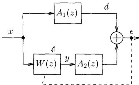
Fig. 2. Adaptive feedforward control.
