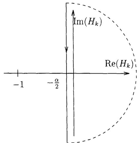
Fig. 8. The Nyquist curve of a resonator channel.
