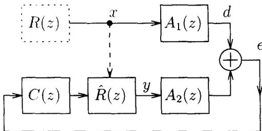
Fig. 4. Resonator based control.
