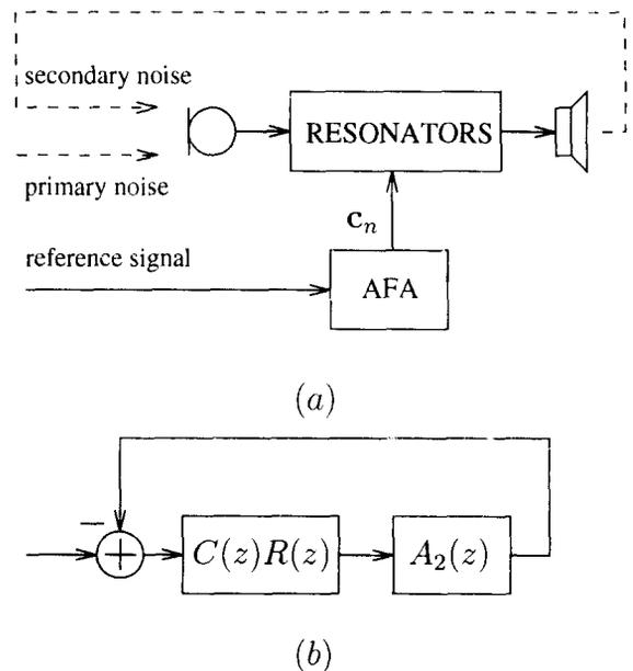
Fig. 7. Periodic noise control: (a) physical arrangement, (b) block diagram of the control loop.
