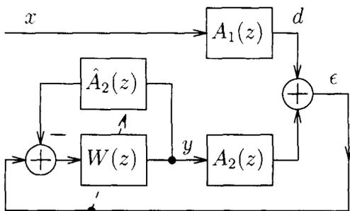
Fig. 1. Adaptive feedback control.
