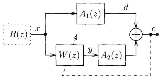
Fig. 3. Feedforward control of periodic noise.
