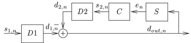
Fig. 2. Active distortion cancellation at the output of the driver.
