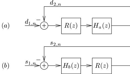
Fig. 6. Simplified block diagrams for stability analysis. Diagram (a) and (b) correspond to Fig. 2 and Fig. 3, respectively.
