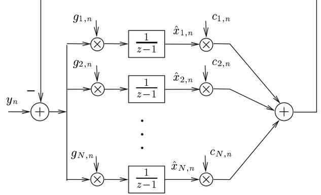
Fig. 4. The resonator based observer.
