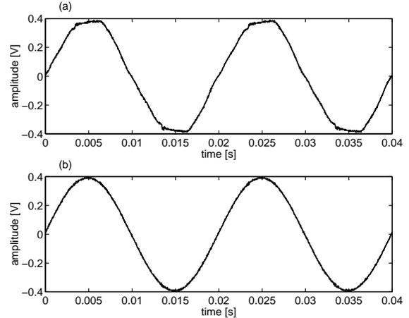
Fig. 10. Sensor voltage waveform without (a) and with (b) distortion cancellation.
