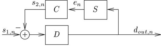
Fig. 3. Active distortion cancelation at the input of the driver.
