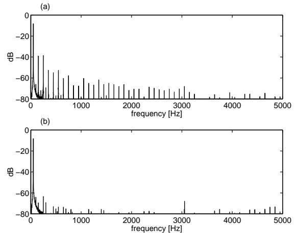
Fig. 11. Spectrum of the sensor voltage without (a) and with (b) distortion cancellation.
