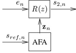
Fig. 5. The controller with the adaptive Fourier analyzer (AFA).
