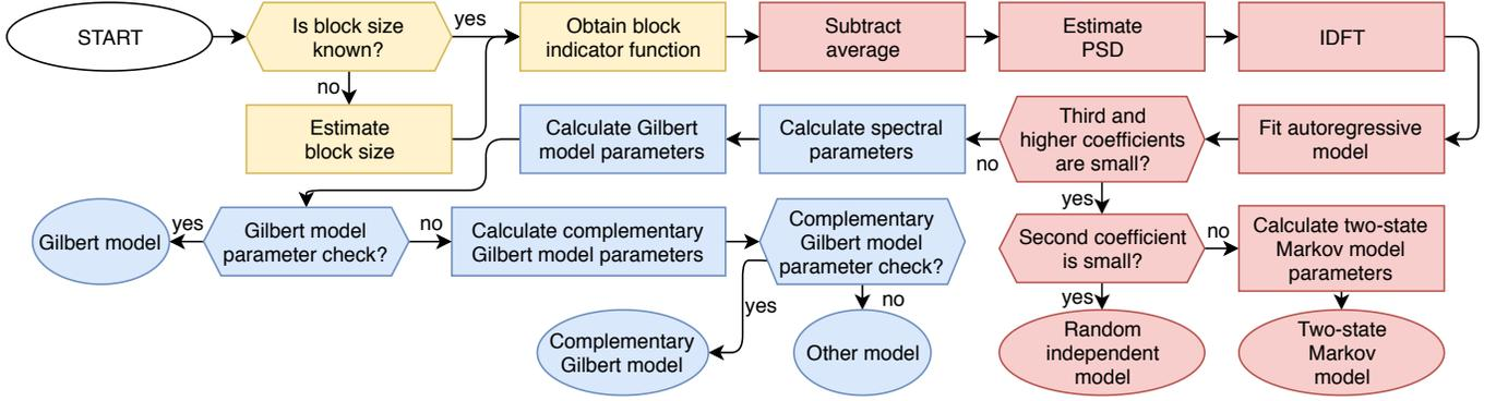
Fig. 3: The proposed identification method
