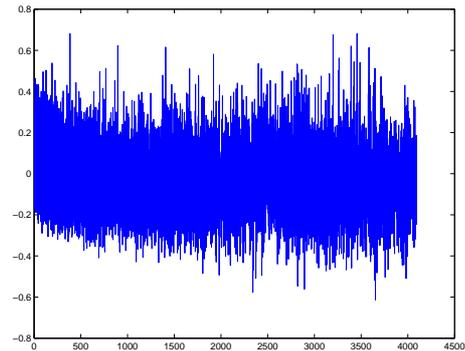
Figure 6: Estimated DNL of the ADC using the result of the ML estimation.
