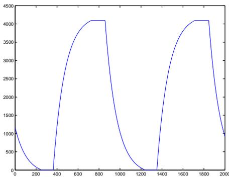
Figure 3: Exponential excitation signal. It contains alternating falling and rising parts.
