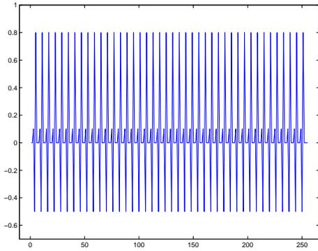
Figure 1: DNL of the simulated ADC as a function of the transition level vector.
